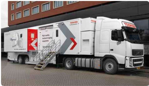
The mobile unit is equipped with a digital leveling system for quick setup on arrival. A patient lift enables easy access also for patients with limited mobility.
