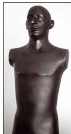
Fig. 2: Anthropomorphic phantom which contains a skeleton and lung-tissue-equivalent material, surrounded by soft-tissue-equivalent material.
