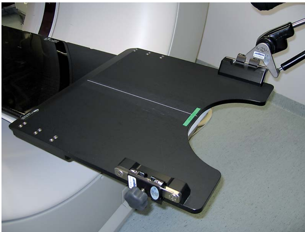
Fig. 2: Foot holder device fixed to CT couch (radiotherapy top). Only one foot support is fixed.
