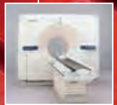
1985 Toshiba introduces the world's first continuously rotating CT scanner with slip-ring technology.
